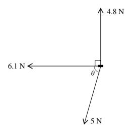
A small block of mass 1.25 kg is on a horizontal surface. Three horizontal forces, with magnitudes and directions as shown in the diagram, are applied to the block. The angle  $\theta$  is such that  $\cos \theta = 0.28$  and  $\sin \theta = 0.96$ . A horizontal frictional force also acts on the block, and the block is in equilibrium.
